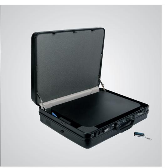
The Jammer is designed for intelligent and permanent counteraction to radio-controlled explosive devices (RCED) and for protection against unauthorized tapping, which is achieved by using special radio means operating in the working frequency range of the Jammer.
